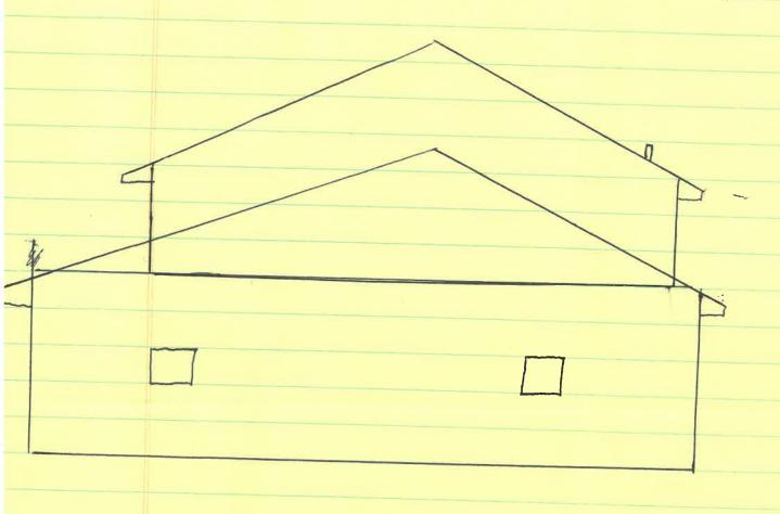
2x6 Rafters 16"0c 2x4 walls 16"0c 2 celetox 5 Roof Sheeting 2x8 floor joist 16"0c
